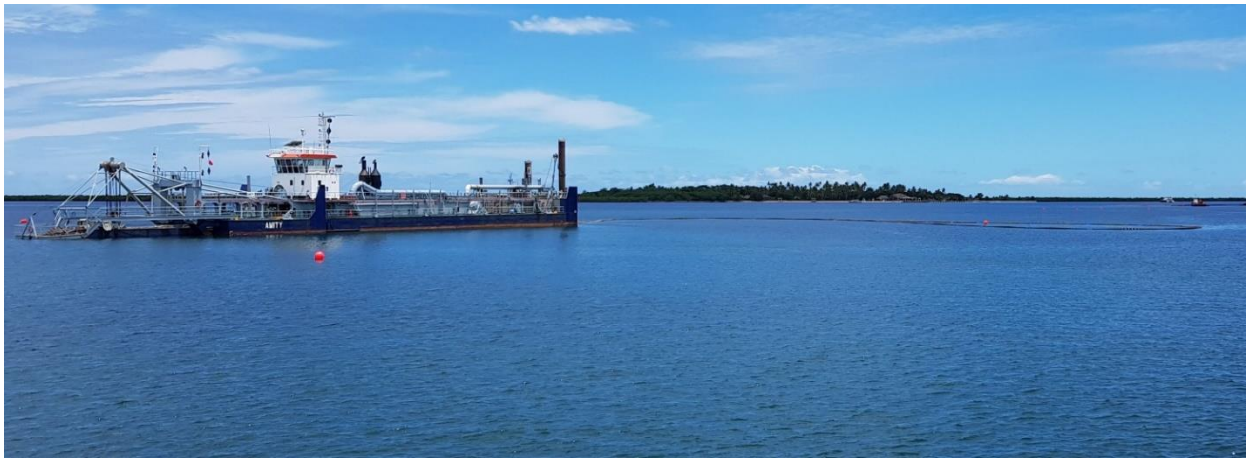
Figure 5 Example of a suction dredge - the AMITY, which has previously done dredging at Funafuti
